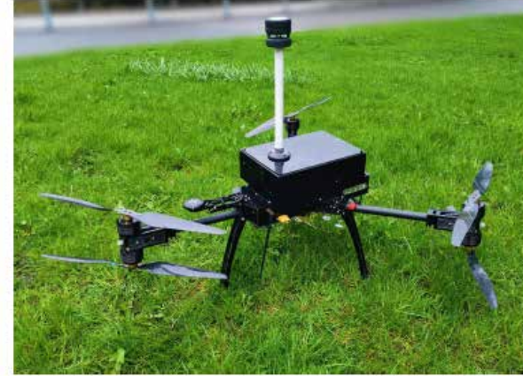
Drone: SkyEye Micro, 1 kg payload, 30 min durability. Sensors: Minisniffer, optical and bag-sampling. Scipper & 4 campaigns 2021 in Nat project
