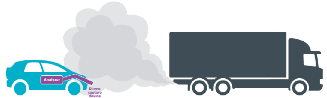
Schematic of plume chasing remote emission sensing device.
